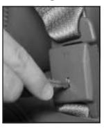
Disconnect the quick release latch plates for the lap shoulder belts on the bench seat to be removed. To do this, press the tip of a key into the release hole of the safety belt buckle while pulling up on the safety belt.
